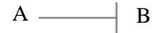
Fig. 3.3. A counteracts the outcome B or the proper working of object B
