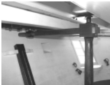
Figure 2: Old-fashioned steering. Rudder stem with tiller on frigate from 1860. The cordage is fastened to the tiller, runs through several cabins and is lead out through the ceiling to the deck where the helm is placed
